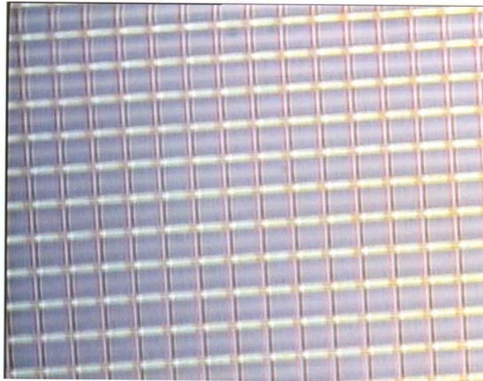
**Figure 3.** Cylindrical microlenses are used to focus light through the ITO electrode.
