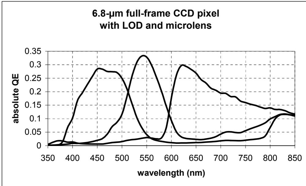
**Figure 6.** Absolute quantum efficiency of a 6.8- $\mu\text{m}$  pixel full frame CCD with color filters and microlens. Measurements were taken with clear (no anti-reflection coating) cover glass in place.
