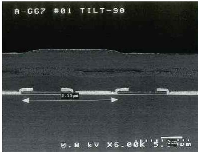
**Figure 1.** The lighter material is the ITO in this scanning electron microscope (SEM) image of a cross section of a 2-phase CCD pixel.
