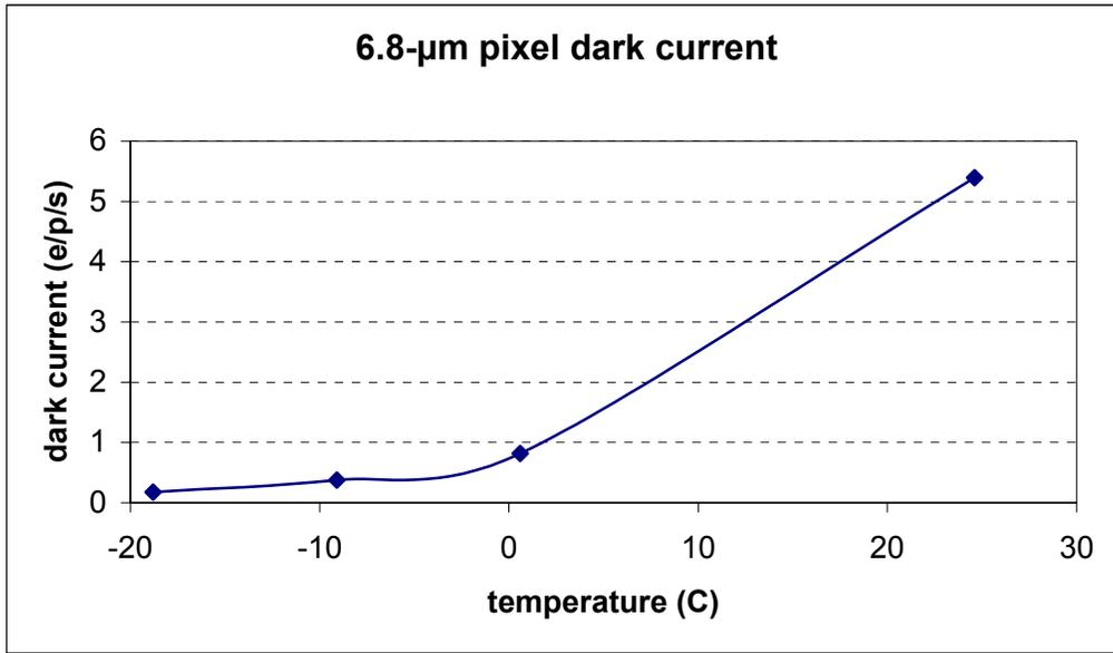
**Figure 8.** This measurement shows a typical dark current of 5.4 e/p/s at 25°C, corresponding to 1.9 pA/cm<sup>2</sup> for the 6.8-µm pixel.
