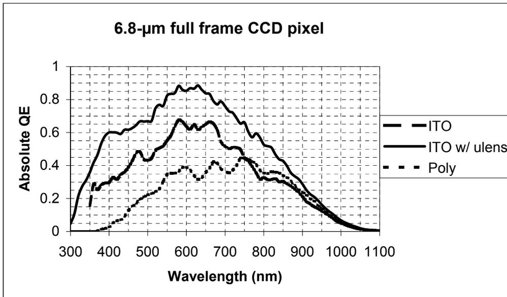
Figure 5. Absolute quantum efficiency of a Kodak 6.8- $\mu\text{m}$  full-frame pixel without coverglass.
