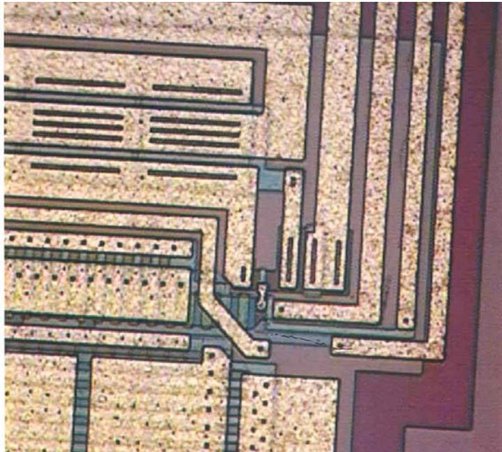
**Figure 7.** The output structure of the KAF-3200ME sensor contains a dual-stage amplifier. In this image, charge is transferred to the right along the horizontal CCD.
