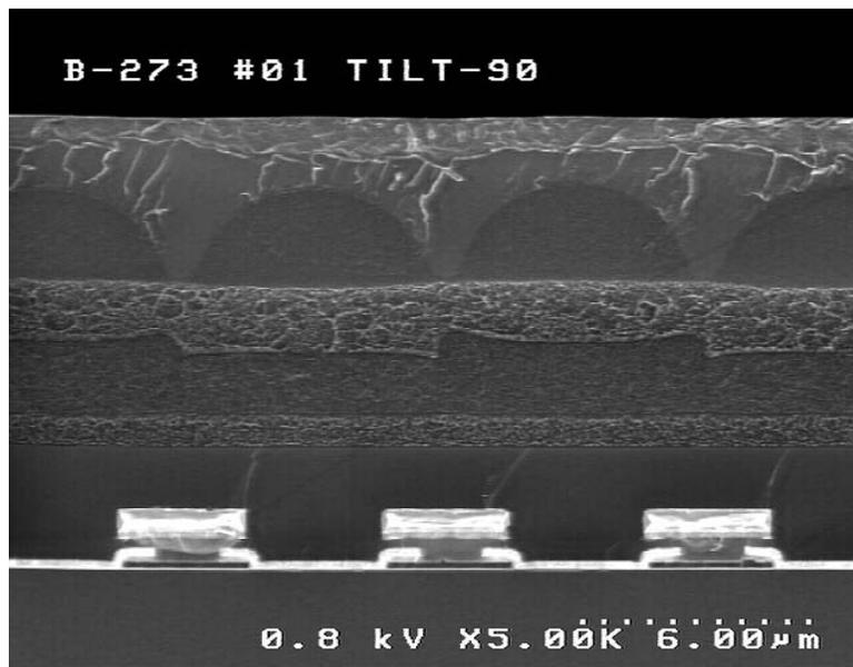
**Figure 4.** For color devices like the Kodak KAF-5101CE image sensor shown here, a metal aperture and traditional lenses are used to reduce color crosstalk. The layer above the microlenses in this image is for protection during dicing.
